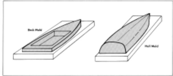
Figure 4. Vacuum Forming Molds
