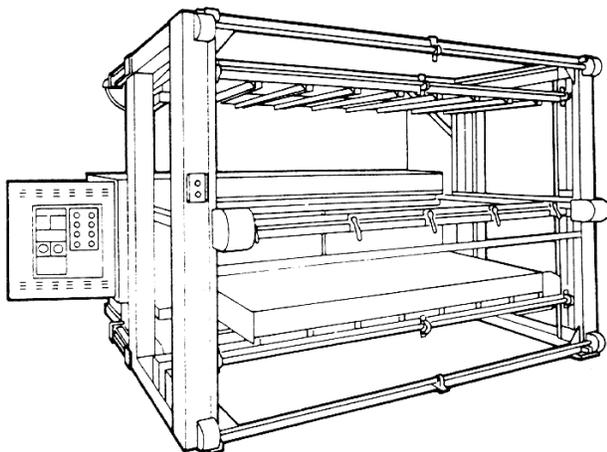
Figure 3. Vacuum Forming Machine
