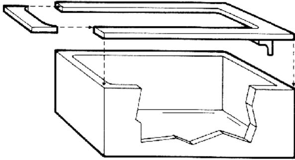
Figure 4. Cast Aluminum Mold
