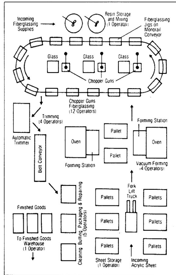
Figure 2. Typical Plant Flow Diagram
